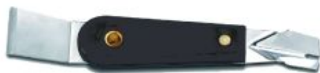
03945 2-in 1 Glazing Tool, High Carbon Steel Blade w/nylon handle. Flat end to clean out old putty and the V-Shape end to apply and smooth new putty.
