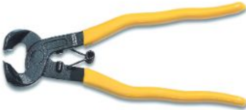
17017 8-1/2" Professional Tile Nipper, Drop Forged. Drop forged carbon steel with top quality and tough carbide tipped jaw. Automatic spring powered reopening function. An ideal nipper for shaping tile to fit around such objects as fixtures, tube, pipes, sinks etc...
