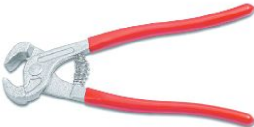
17018 10" Quarry Tile Nipper, Drop Forged. Professional design for easy work with hard and thick materials. The center style jaws are both straight and 5/8" wide. They open to a full 2" for ease of entry. Both jaws are tipped with a special carbide that resists chipping and breakage. Plastic grips are supplied on the strong steel forged handle.
